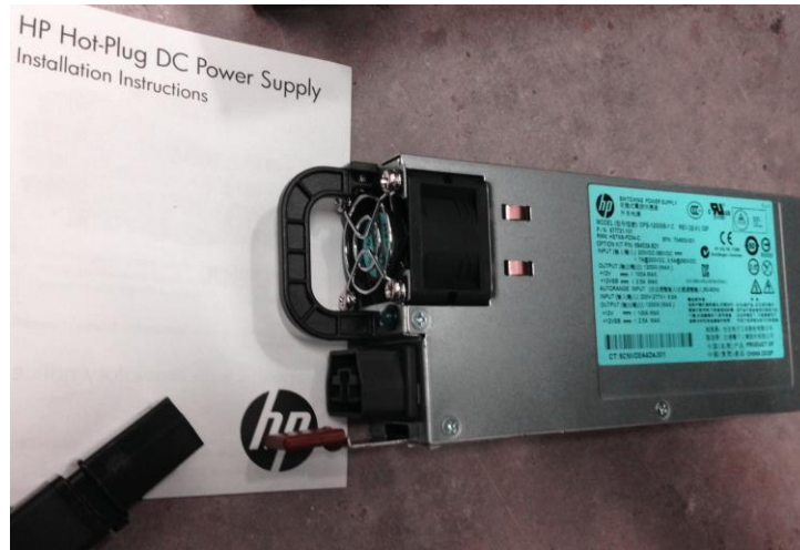
Figure 2 – 380v dc HP Common Slot power supply
